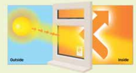
Stage 2. With heat now in the building, the inner pane of Pilkington K Glass™ acts to prevent energy loss back out of the window unit.
